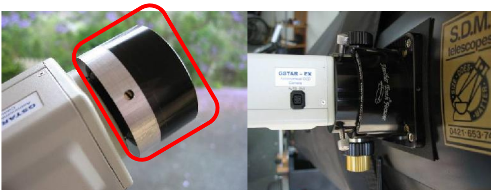
Machined 2" adaptor used to get focus in a low profile focuser on a 20" Dobsonian designed for visual work
