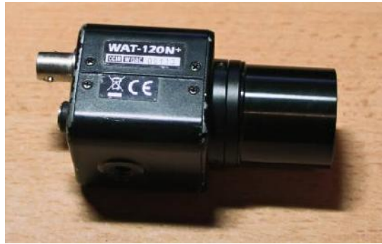
Watec camera mated to a high quality C-1.25" nosepiece
